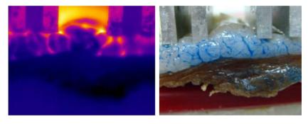
**Figure 3** Lt. four phase-controlled sources of RF (multisource RF technology) used on *ex vivo* duck tissue demonstrating a selective heat flow through the dermis and the fibrous tissue surrounding the subcutaneous fat lobules. Rt. Tissue stained with Aniline Blue reveals a match between collagen fibers network (stained in blue) and the heating pattern on the left side.
