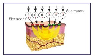
**Figure 1** Typical multisource RF configuration uses six independent phase-controlled RF generators. For skin tightening and body contouring, the three generators on the left will be configured to "plus" and the three on the right to be "minus".
