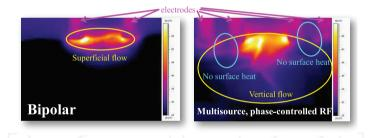
**Figure 5.** Comparison of bipolar vs. multisource phase-controlled RF system. With bipolar device (300 W, 1 s), superficial flow of energy, penetrates only to 1.5 mm depth. Multisource phase-controlled RF system (4 electrode,  $2 \times 150$  W, 1 s) shows vertical flow of energy, penetrates to 6 mm depth. Absolutely no surface heat between the external electrodes. The surface flow is only between the two middle electrodes.
